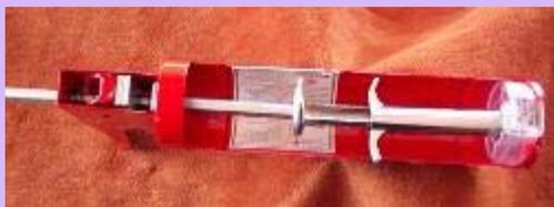
For anyone wanting to make a clay/caulk gun adapter disk, cut a 2 inch circle out of at least 3/4" thick wood. Drill 2/3 of the way through the center with a 7/8" drill bit. Then drill the rest of the way through the center with a 5/8" drill bit. If you have a tube of caulk, trace around it for the perfect size for your cut line, unless you have a 2" circle cutter for a drill press, which is easier yet.
