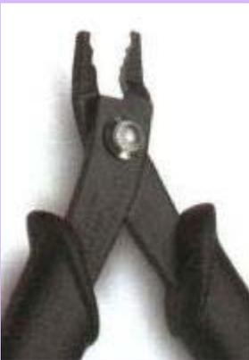
**Crimpers:** Crimpers are designed to crimp crimp beads into a round form, instead of squishing them, as regular pliers do.
