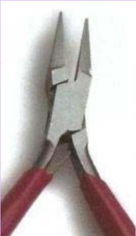
**Flat/bent nose pliers:** Flat or bent nose pliers are designed to hold wire firmly and to make sharp bends and right angles with wire. They come with serrated and non-serrated faces. Serrated faces have a stronger grip, but non-serrated faces don't leave any marks.
