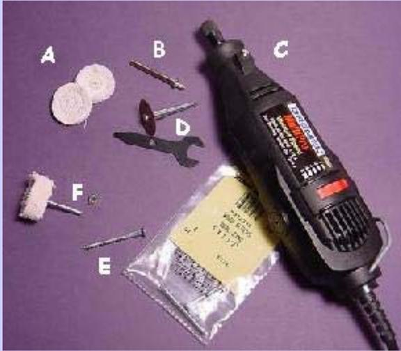
The key drawback (IMHO) with the Dremel, however, is it's tiny cloth polishing wheel, a thin little disc that's about 3/8th inch thick and 1 inch in diameter (A). The area that actually touches the item to be polished ends up being very small -- too small for my needs.
